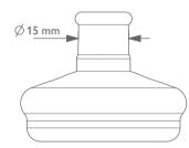
Pressure release valve: Upright has a pressure release valve ("pop-off") which limits the airway pressure to  $30-45 \text{ cmH}_2\text{O.A}$  hissing sound can be heard when the valve opens. If higher airway pressure is needed, press downwards on the valve with the index finger while squeezing the bag.
