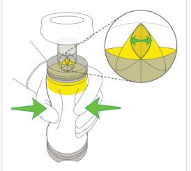
Squeeze the bag. Check that the yellow valve opens and closes with every squeeze.
