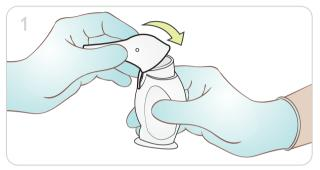
Reattach the head, ensuring a complete seal with the body.
